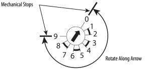
**IMPORTANT** Adjust the switches gently and do not turn past the mechanical stops.
