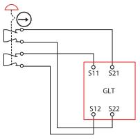
When only one dual-channel E-stop button is used, the maximum safety performance rating is Cat 4 PLe and SIL CL3.
