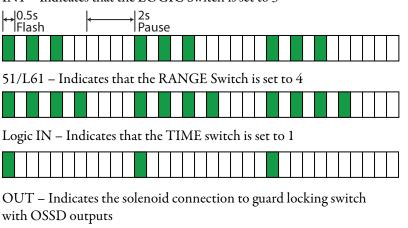
5. Cycle the power to the GLT safety relay. After power-up, the current switch settings are compared to the values in the EEPROM, and the input and output circuits are checked. Upon successful completion of the internal checks, the GLT safety relay is ready for operation.
