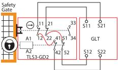
Since the TLS3-GD2 interlock switch has multiple contacts in series, the maximum safety performance rating is Cat 3 PLd and SIL CL2.
