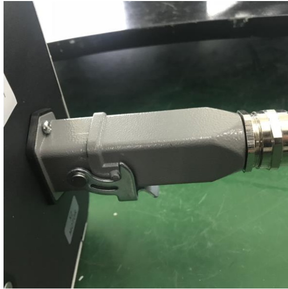
Figure 4.3 Connect controller and robot by heavy-duty cables
