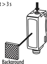
Align the sensor to the background. Press and hold button for three seconds until yellow LED starts flashing. Release the button. The first condition has now been taught.
