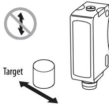
**IMPORTANT** Due to the detection method, targets traveling horizontally to the sensor optics are detected. Targets that travel vertically cannot be accurately detected. For more dependable background suppression, a minimum separation distance is recommended between the target and the background.
