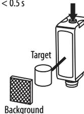
Insert the target between the sensor and the background. Press and release the button. The teach process is complete.
