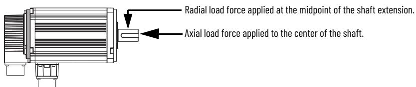
The following tables represent 40,000-hour  $L_{10}$  bearing fatigue life at various loads and speeds. This 40,000-hour bearing life does not account for possible application-specific life reduction, such as bearing grease contamination from external sources.
